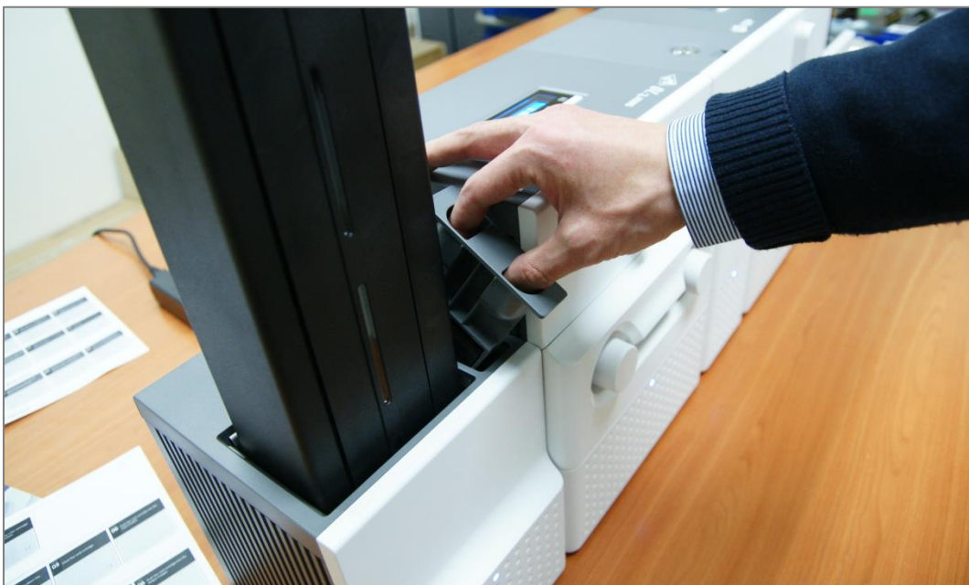
Figure 27 Detachment of disposable cleaning roller holder
