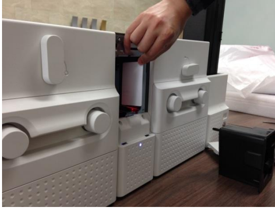
Figure 125 Card jam in Hybrid Flipper 4
