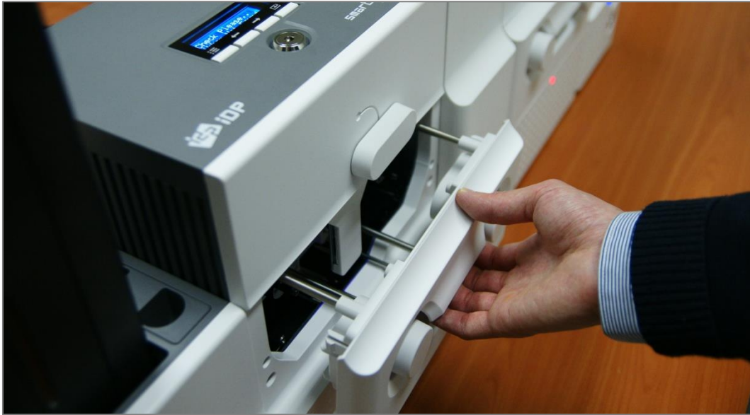
Figure 20 Pulling out ribbon / film cartridge
