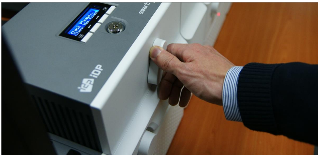
Figure 19 Ribbon / film cartridge unlocking
