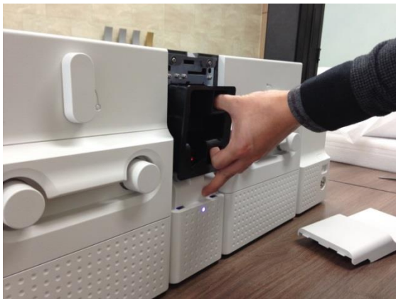
Figure 123 Card jam in Hybrid Flipper 2
