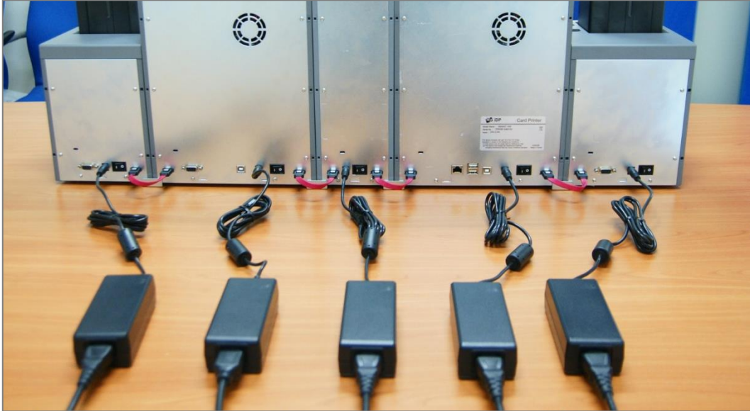
Figure 57 Cable connection of SMART-70 IPHLO
