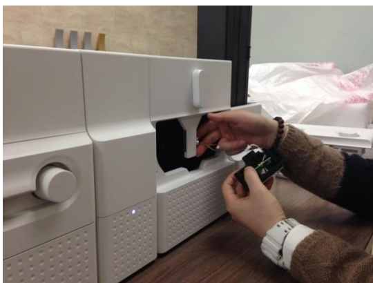
Figure 161 Laminator Head replacement 5
