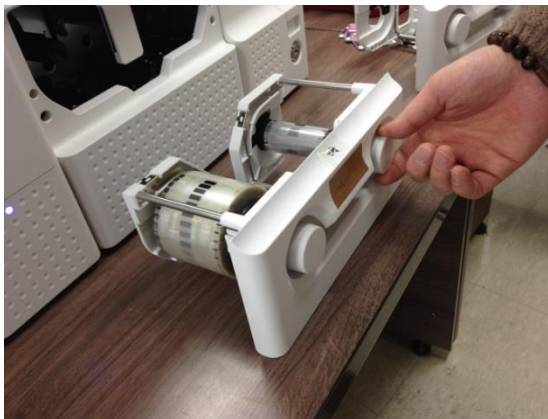
Figure 130 Card jam in Laminator 5
