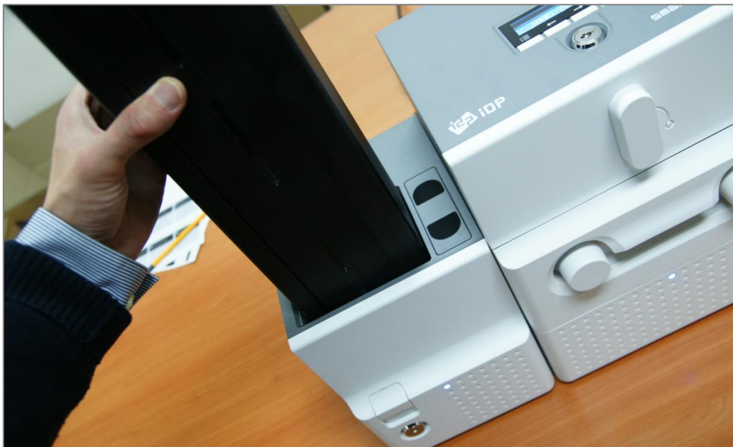
Figure 39 Loading card cartridge into Input Hopper
