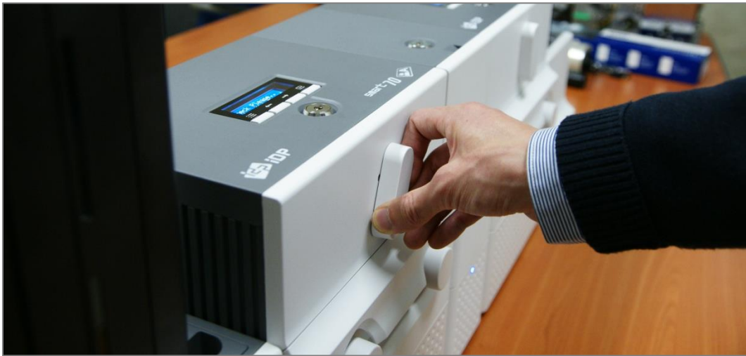
Figure 26 Ribbon / film cartridge locking
