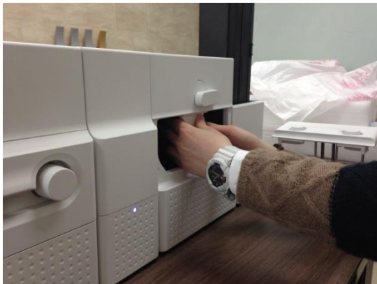
Figure 159 Laminator Head replacement 3
