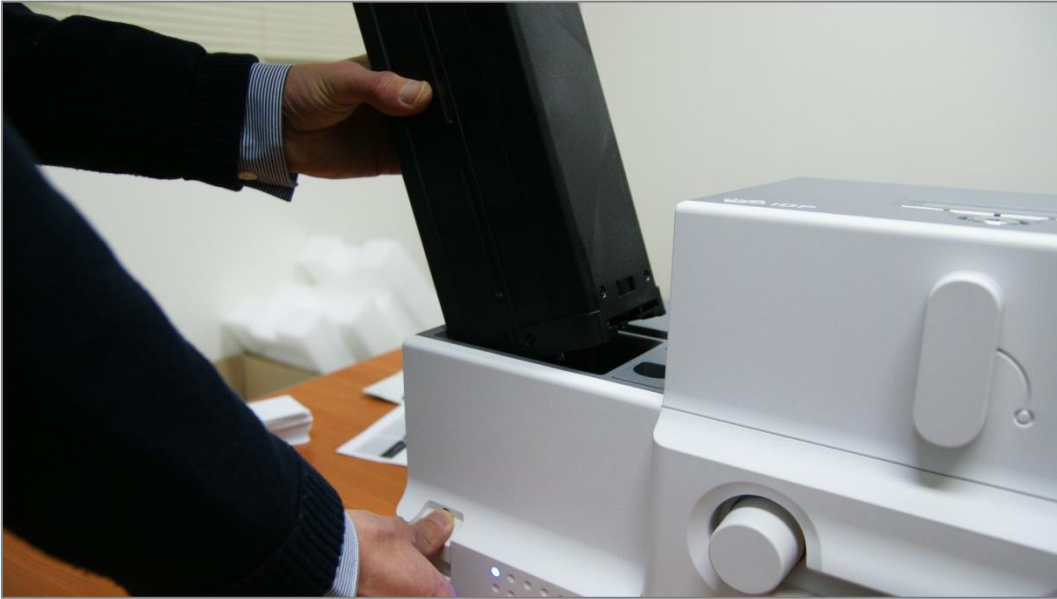
Figure 32 Card cartridge release from Input Hopper
