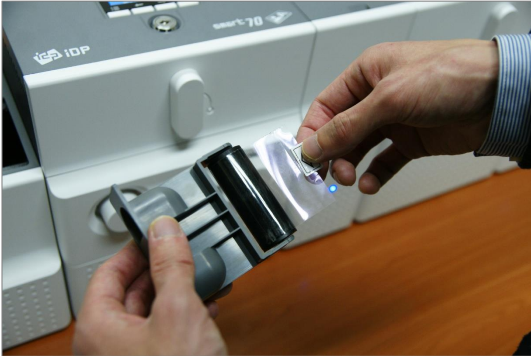
Figure 30 Removal of new disposable cleaning roller protector
