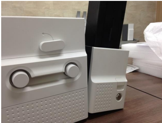
Figure 131 Card jam in Output Hopper 1
