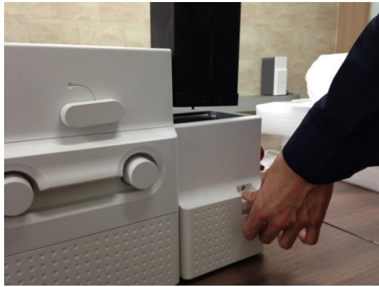
Figure 149 Output Hopper cleaning 2
