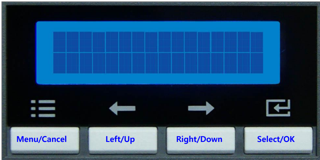
Figure 11 Control panel of Laminator
