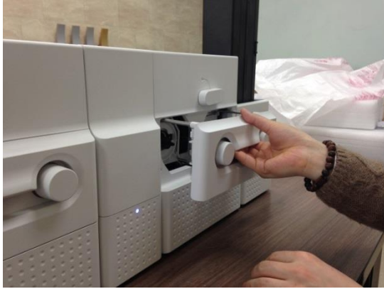
Figure 158 Laminator Head replacement 2
