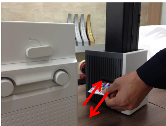
Figure 133 Card jam in Output Hopper 3
