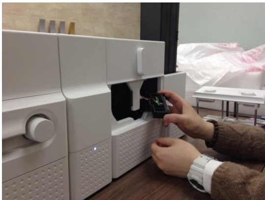
Figure 160 Laminator Head replacement 4
