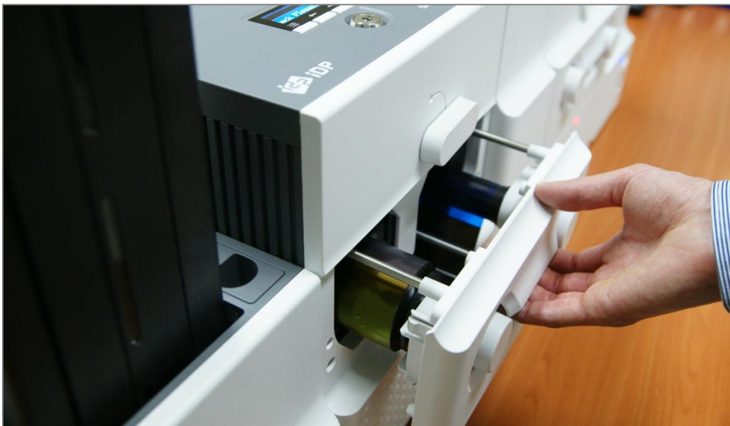
Figure 25 Ribbon / film cartridge insertion
