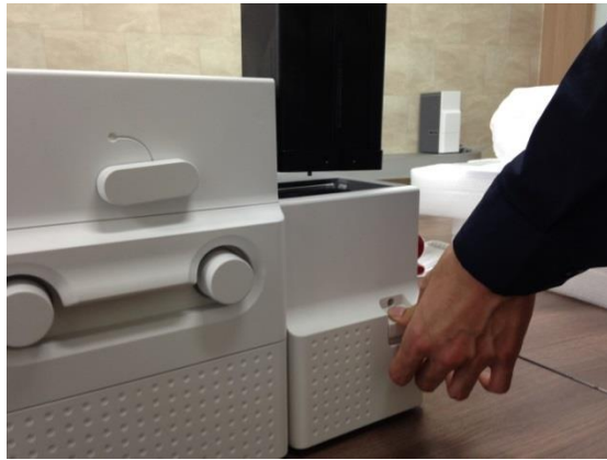
Figure 134 Card jam in Output Hopper 4
