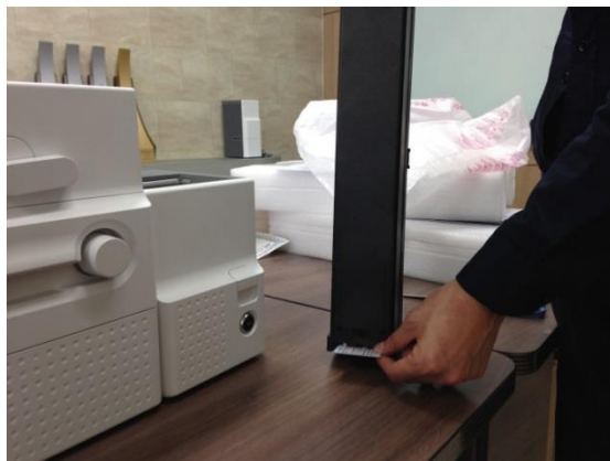
Figure 135 Card jam in Output Hopper 5
