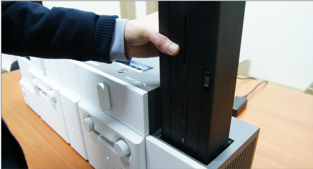
Figure 40 Loading card cartridge into Output Hopper
