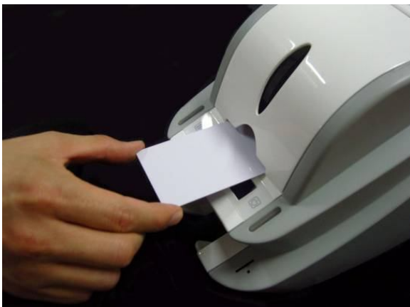
Pic.24 Loading the cards 3
