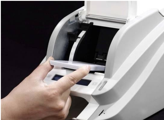
Pic.23 Loading the cards 2
