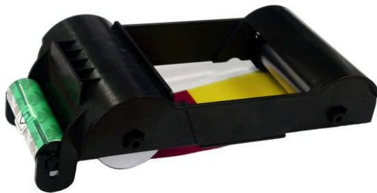
Pic.15 Installing the cleaning roller
