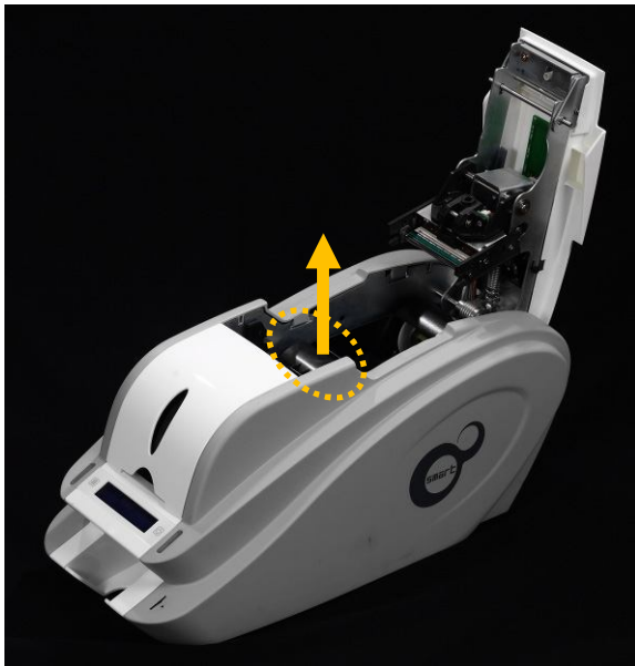
Pic.12 Take out the ribbon cartridge
