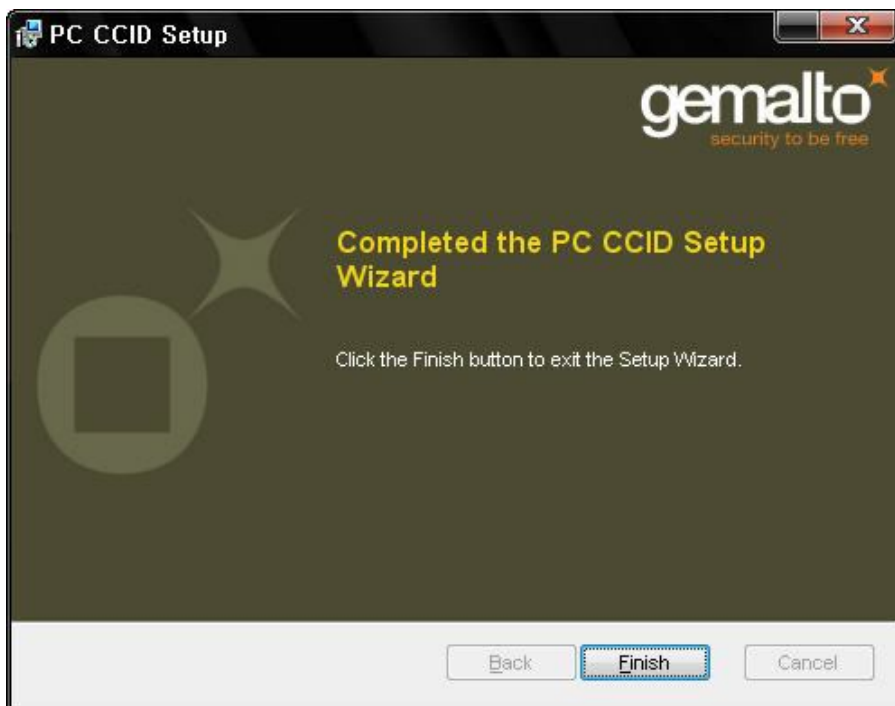
Pic.128 Completing the smartcard reader driver installation
