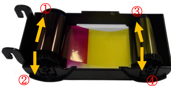
Pic.14 Loading the ribbon 2
