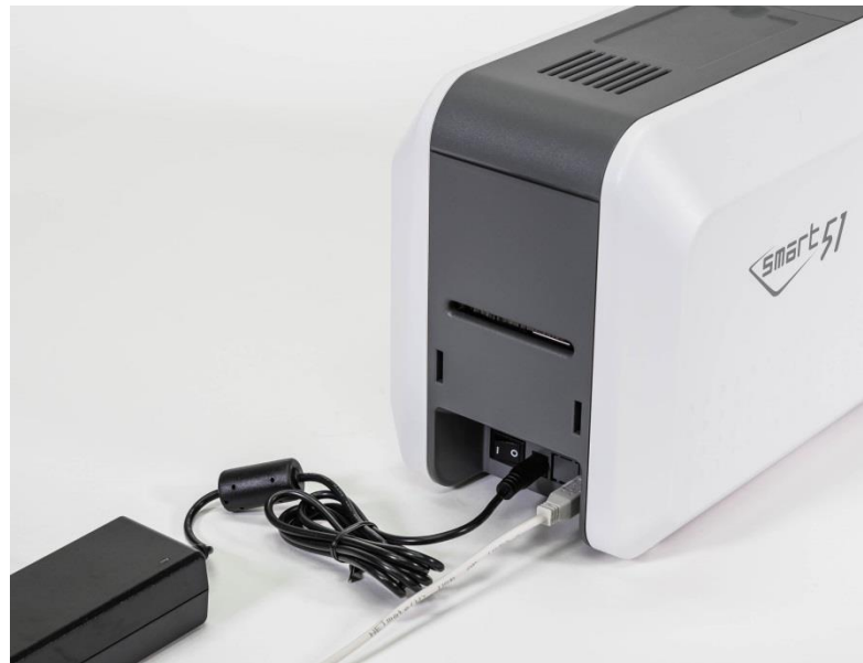
Figure 9 SMART-51S Connection of power and USB cable
